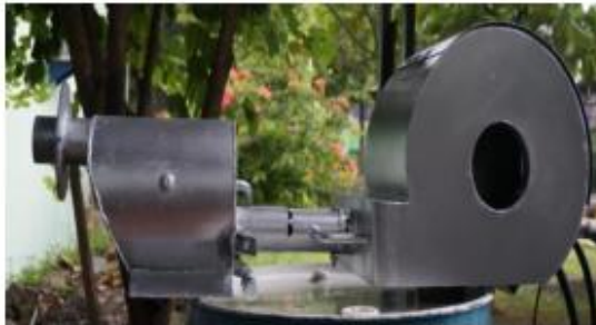
Figure 2. Aluminum Melting Stove with 5 kg Capacity Using a Combination of Vaporizing and Air Atomizing Burners with Waste Oil Fuel
