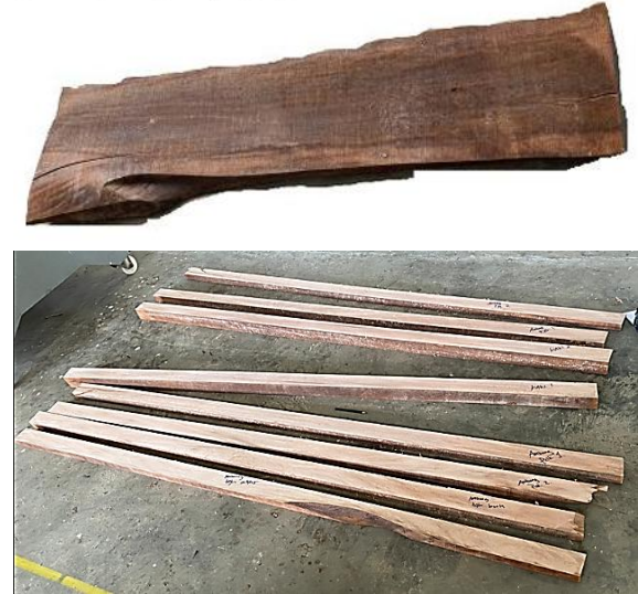
Fig. 1 Cutting Using Ripsaw
