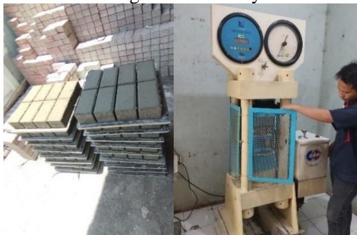
Figure 2. Paving block compressive strength testing
