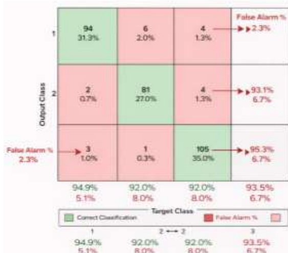
Figure 4. Confusion matrix of the ANN classification results for the three engine operating conditions: Normal, Degraded, and Faulty.
