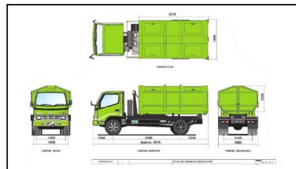
Figure 2. Specification of truck (Spesifikasi Teknis pengadaan Arm Roll Kontainer, 2012)
