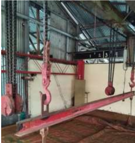
Figure 5. Ice Block Crane/Lifter
