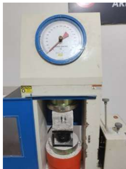
Figure 1. Compressive Strength Test Using Hydraulic Loading
