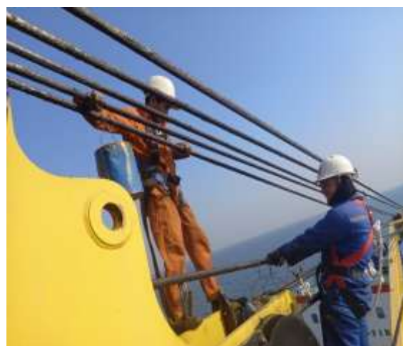
Figure 1. Re-greasing Wire rope Deck crane
