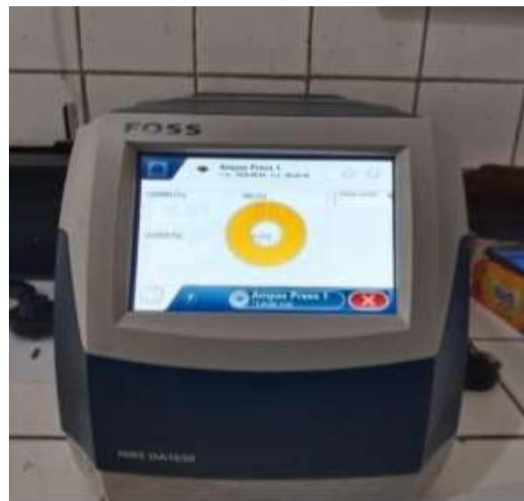
Figure 4. FOSS NIRS DA1650 instrument used for routine measurement of oil, moisture, and non-oil solids in press fibre.
