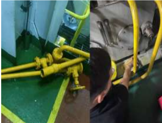
Figure 3. Hydraulic Steering Gear System Piping
