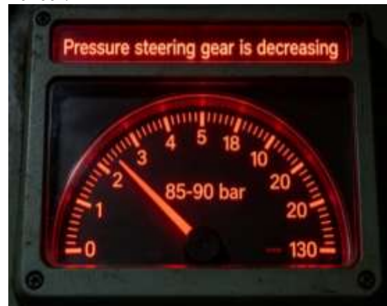
Figure 2. Steering Gear Hydraulic Pressure Condition
