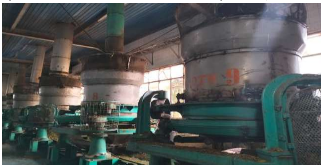
Figure 1. Open Top Roller (OTR) machine used in the black tea leaf rolling process at PTPN IV Bah Butong Unit.
