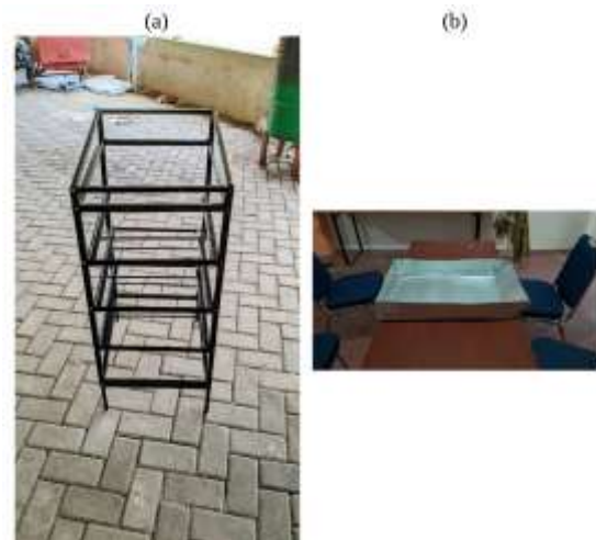
Figure 3. Fabrication: (a) welded hollow-steel frame and (b) zinc galvanized biopond.
